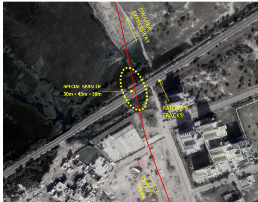
FIGURE 5.17: LOCATION OF SPECIAL SPAN AT RAILWAY TRACKS
